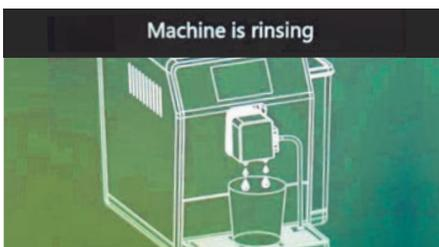
The appliance starts the rinsing stage of the internal circuits and waste water is dispensed from the coffee dispensing spout. The display of the appliance shows the appropriate screen.
