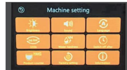
When using the appliance for the first time or after resetting to factory settings, the appliance language, unit of measurement and water hardness must be set up.
