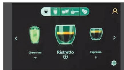
Press the BEVERAGE PARAMETERS button (⊕) to access the relevant beverage parameters.
