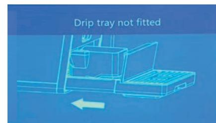
Insert the drip tray into its seat at the base of the appliance.
